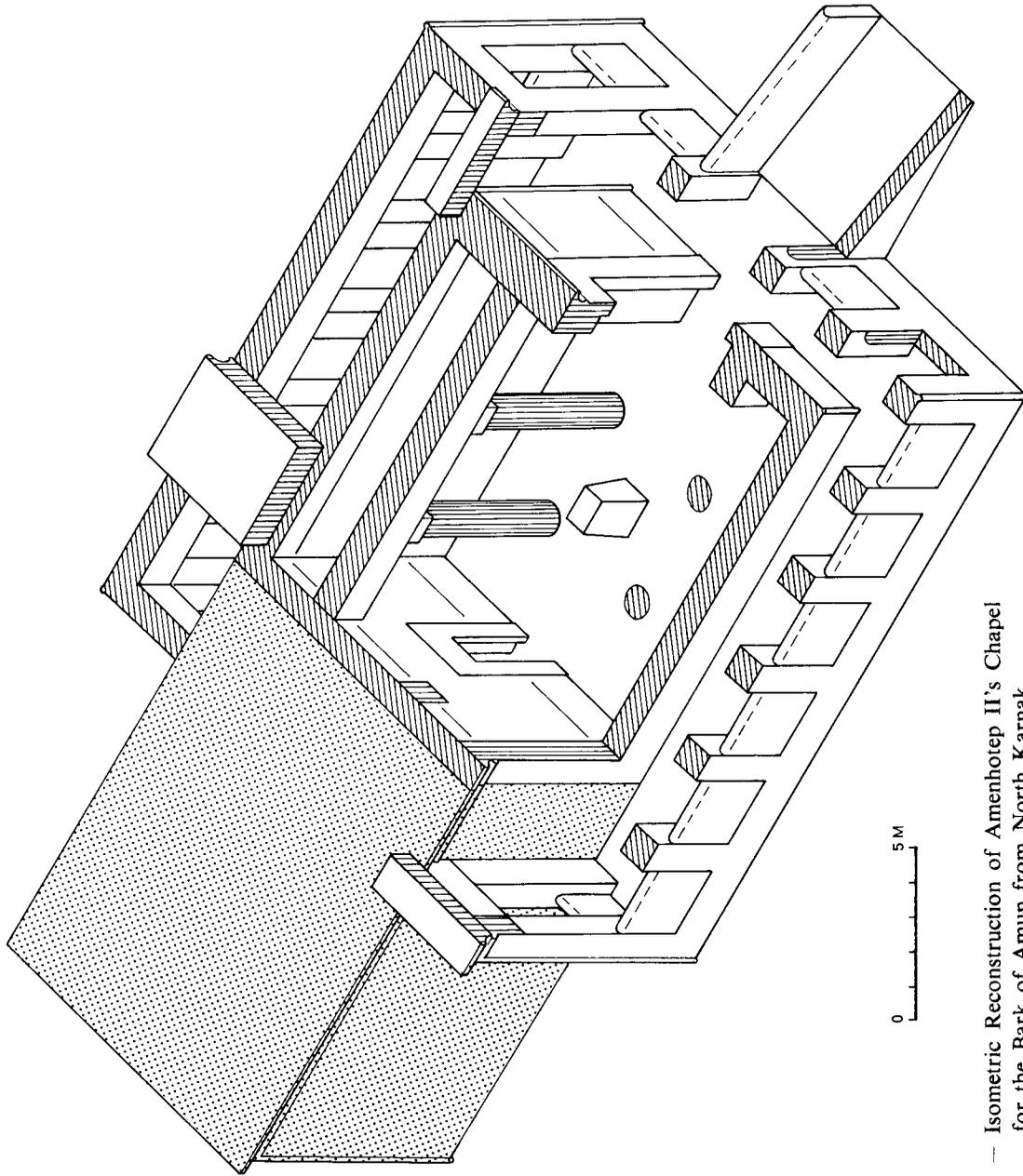
Fig. 1. — Isometric Reconstruction of Amenhotep II's Chapel for the Bark of Amun from North Karnak.
