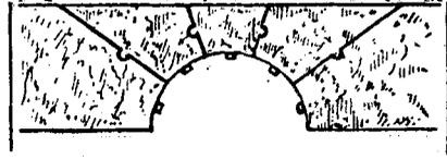
Fig. 13. — QAŞR AL-MUDAKKHIN : Arch with joggled joints counterfeited (from BUTLER, *Ancient Architecture in Northern Syria*).
