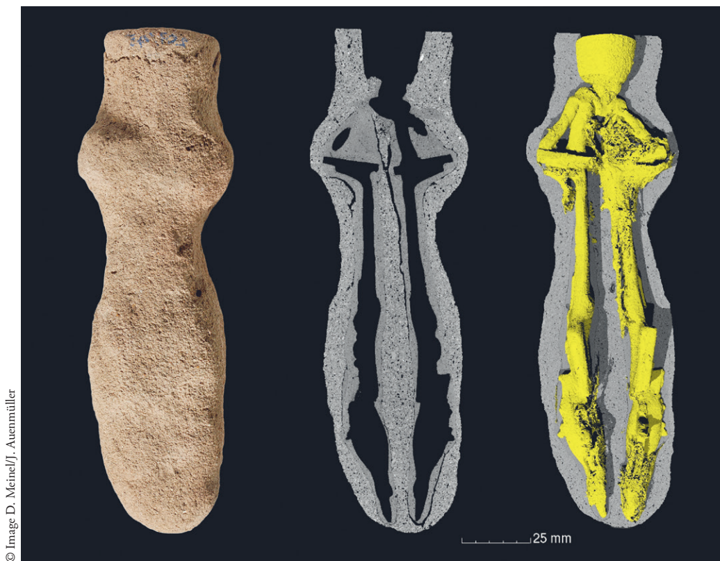
FIG. 1. View, \mu CT-section and \mu CT 3D-reconstruction of casting mould BoS QH 207/45. The mould for casting two Osiris statuettes was never used. It is oriented in the pouring direction, the pouring cup with the gating system is above, the two Osiris figures are upside down. The inner cavity and adjoining cracks are digitally rendered with a coloured fill.
