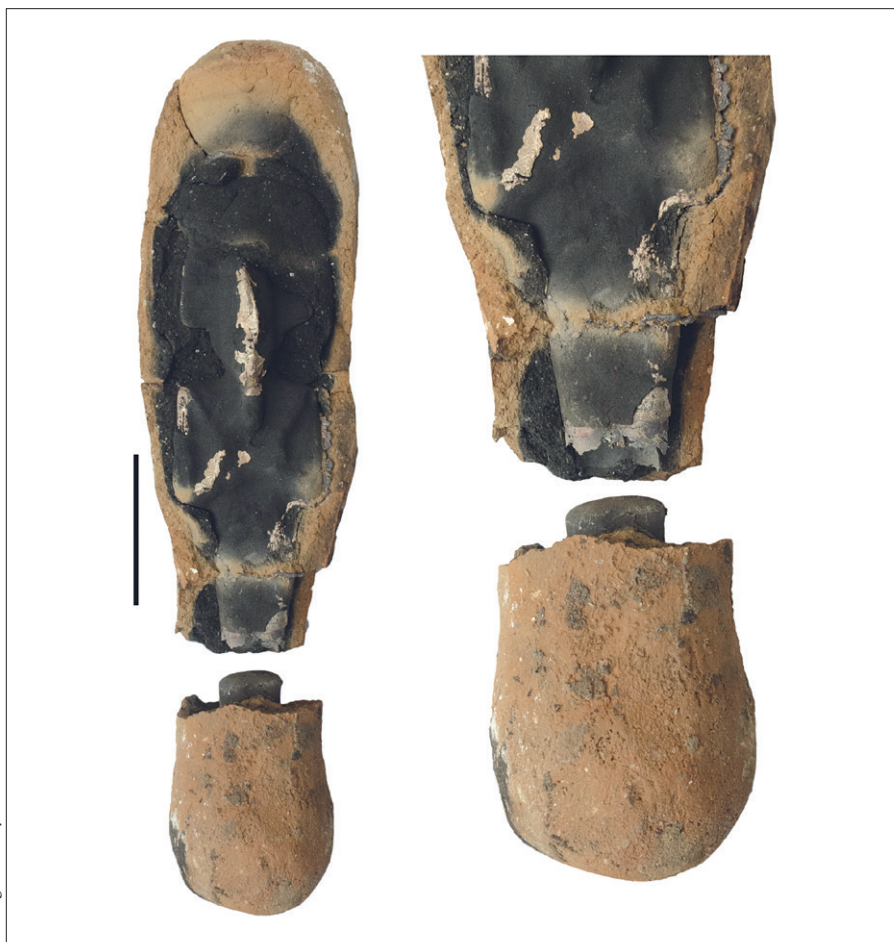
FIG. 15. The figure of Osiris (cf. Figs 11–13) breaks in two during the opening of the experimental mould at the former joint of the wax and the metal. Scale bar corresponds to 5 cm.
