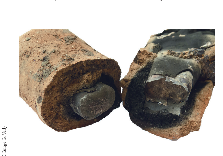
FIG. 16. Detail photography: no fusing occurred between the two parts in any of the experiments.
