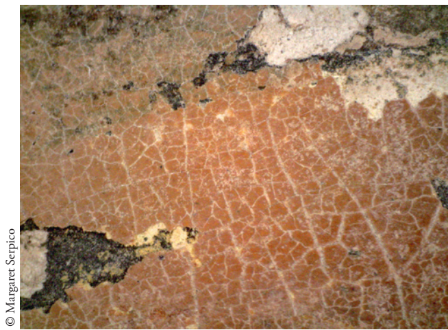
FIG. 14. Coffin of Bakiset, DEM_19_217_093. a. Example of yellow varnish covered with a thin coating of mud on the proper right side of lid, lower shoulder area. Photograph at \times 42.1 magnification; b. Example of yellow varnish displaying craquelure and disengaging completely from the surface on the proper right side of lid, lower shoulder area. Photograph at \times 42.9 magnification.
