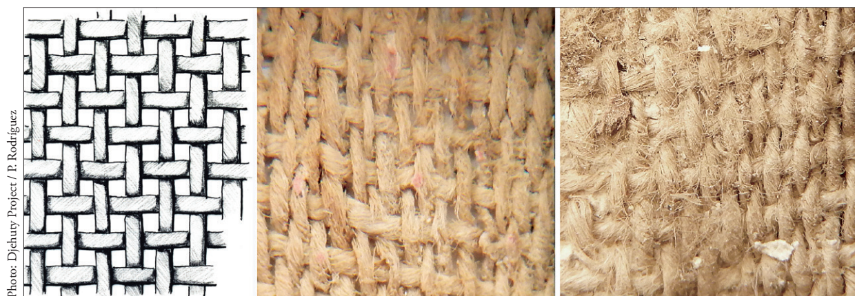
FIG. 7. Detail of the yarns and their densities in the shroud.
