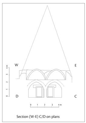
FIG. 9: Bir el-Shaghala Tomb I, east-west section of the two floors with the pyramid restored.
