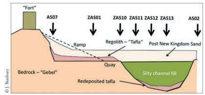
Fig. 25. Proposed cross-section of the ramp and quay showing the locations of boreholes used to construct the section ASO2 and ASO7 bored by E. Hughes in the 2009 season and the remainder by the current authors.
