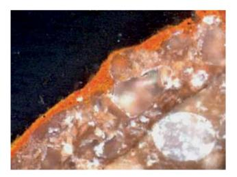
**FIG. 11.** Cross section microscopic image for the painted layer from the north wall, representing the fresco paint layer indicated by the orange pigment integrated inside the paint layer (B. Geahd, 2010).
