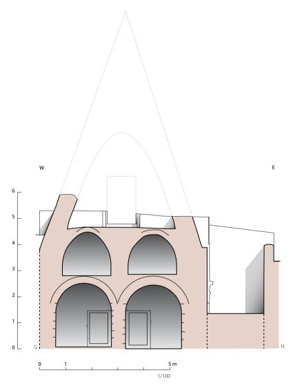
FIG. 10. Section W/E (G-H on plans), 1/100.
