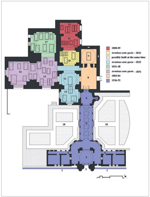
Fig. 2. Plan of Ḥūš al-Bāšā indicating building chronology:
