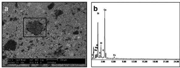
Fig. 6a. BSE image of veined red sample, the square illustrates the grain represented calcium silicate hydrate phase.
