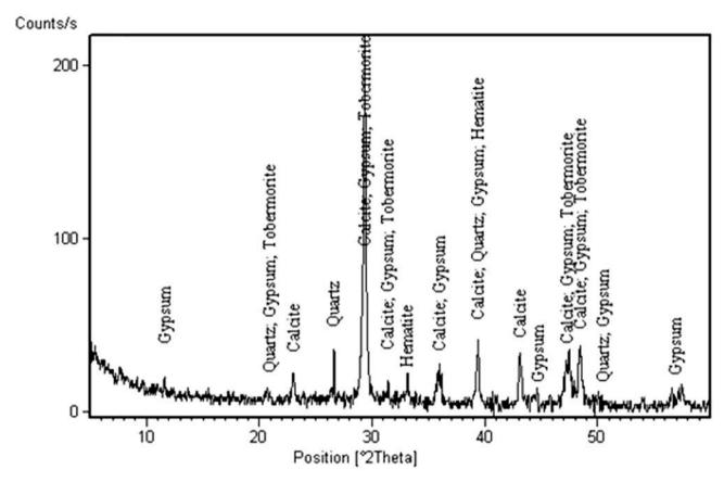
Fig. 7. The XRD pattern of the veined red sample of Sa'id Ḥalīm palace.
