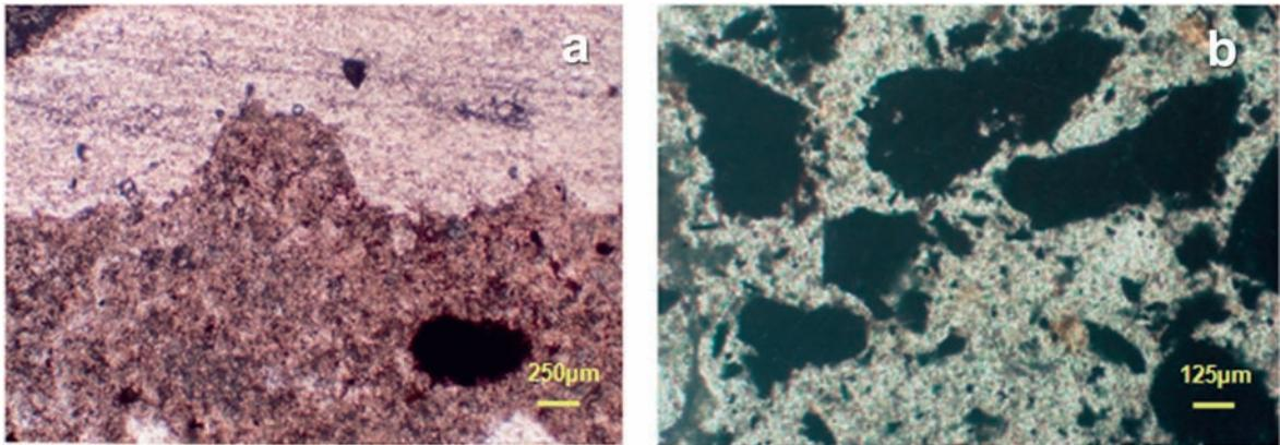
Fig. 5a. The thin cross section image of the veined red sample of Sa'īd Ḥalīm Palace under plane polarised light × 10.
