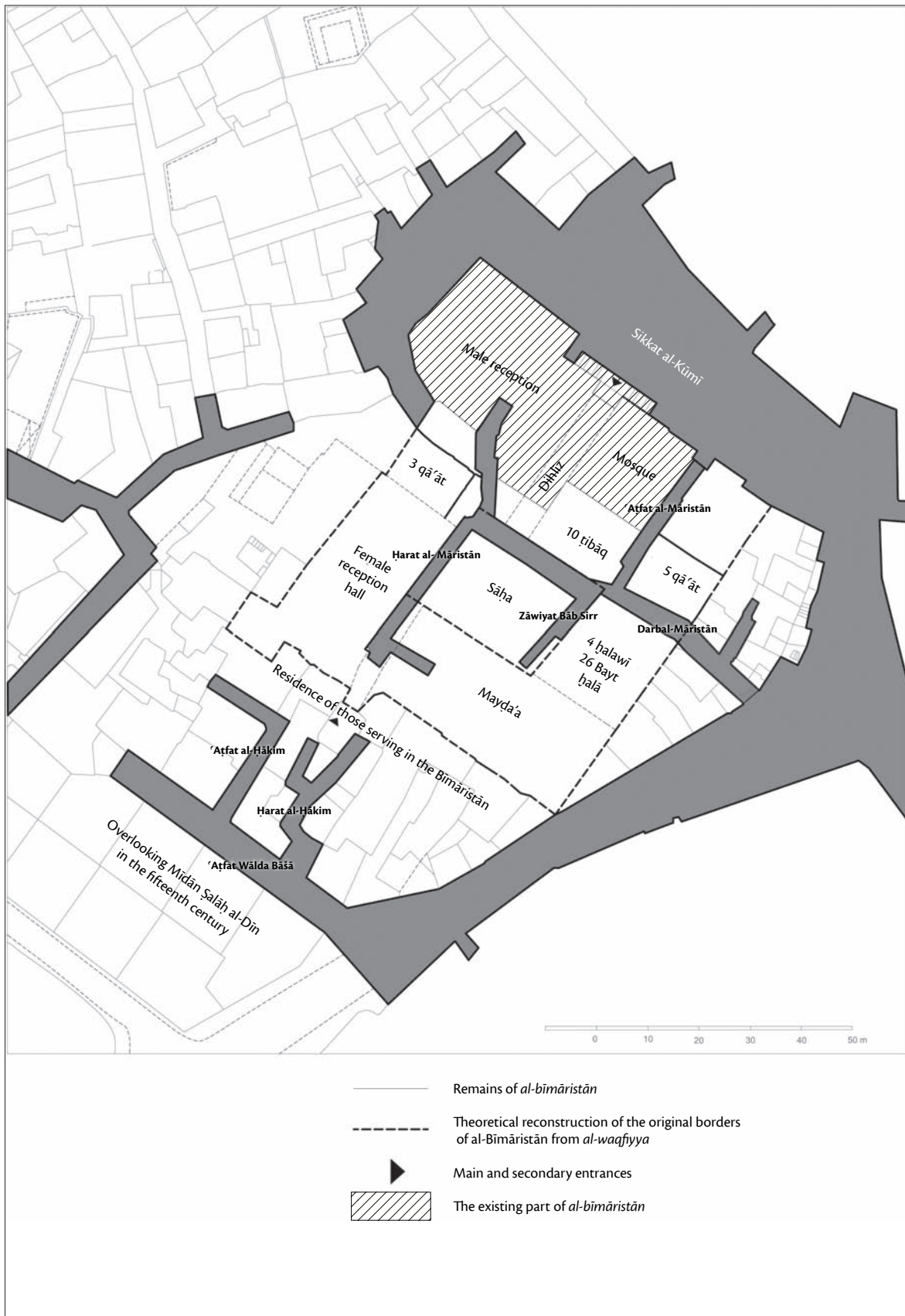
Fig. 5. The remains of al-Bimāristān al-Mu'ayyadī with the actual street pattern around it on which, a theoretical reconstruction of the original borders and internal spaces of the Bimāristān are juxtaposed according to the information recruited from al-waqfiyya of al-Mu'ayyad.
