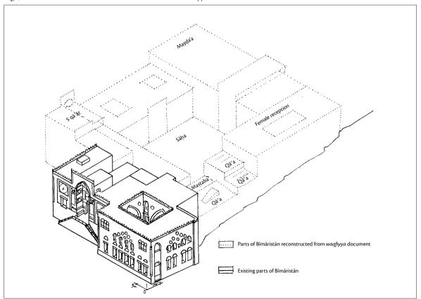
Fig. 8. Isometric view of the remains of al-Bīmāristān al-Mu'ayyadī with a theoretical reconstruction of its original spaces according to the details mentioned in the *waqfiyya*.
