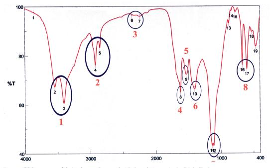
$\label{eq:Fig.10.FTIR} \textbf{FIIR} \ \text{spectrum of the binding medium used with the red pigment in the Sabil Alkazlar}.$
