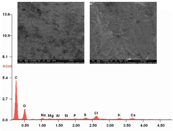
Fig. 7. SEM-EDAX spectra and micrographs of the studied golden pigment from the Sabil Alkazlar. The micrographs show the presence of blisters which can be explained due to hammering of gold leafs.
