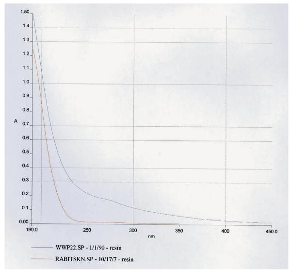
Fig. 12. UV spectrum of the binding medium used with the red pigment in the Sabil Alkazlar, proves that it is rabbit skin glue. [1] Analyzed sample.
