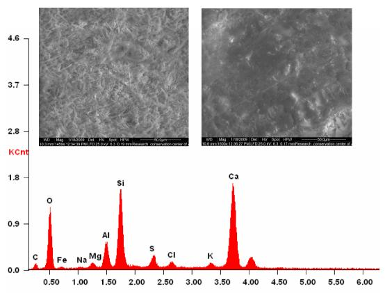
Fig. 3. SEM-EDAX spectra and micrographs of the studied plaster sample from the Sabil Alkazlar. The micrograph (left) shows the gypsum crystals which are the main components of the plaster, while the micrograph (right) shows the growth of anhydrite and halite crystals inside gypsum.
