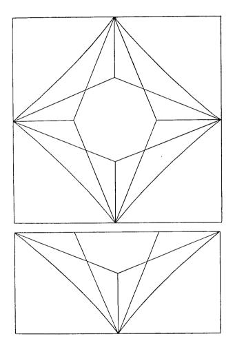
Fig. 2. — Cross-Vault of the squinch.
